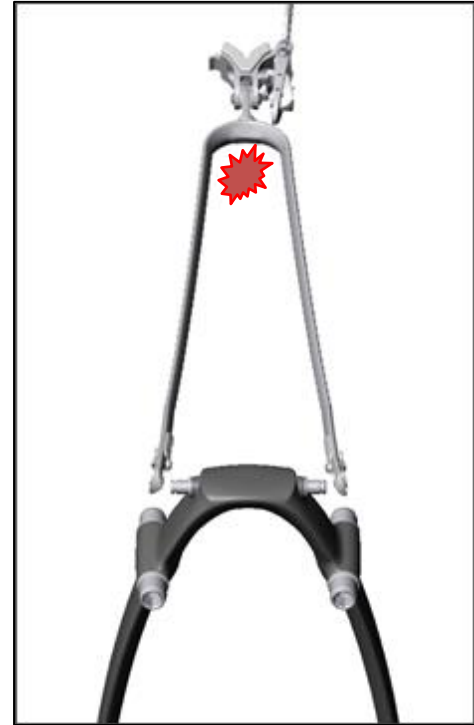
3. Do not over extend the top stay arms. This can damage the top stay.
